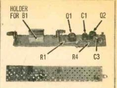
Components are mounted on perf-board as shown. Completed assembly then slides into casing.
