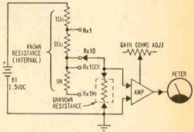
Resistance measuring circuit of FETVM is conventional providing six ranges to read from 10 ohms to 10 megohms center scale.
