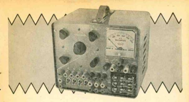
fraction of an ohm to more than 3700 ohms, with a power rating throughout in excess of 25 watts. Other features include built-in current-monitoring meter, fuses, and sufficient banana plug tie-points in the string of power resistors to provide a variety of series, series/parallel, and parallel connections.
