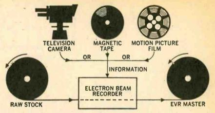
EVR electron beam recorder takes program from TV camera, magnetic tape, or film and generates a master which can be in either color or black and white.
