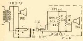
Wire up the jack on the back of the set according to the schematic. The extension speaker, in the dotted lines, is pre-wired.
