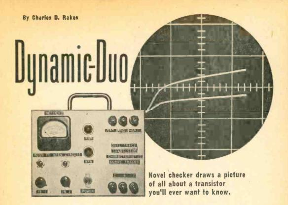
Dynamic Duo is a perfect name for our dual-trace transistor characteristic curve tracer. With this simple tester you can adjust and observe two  $I_c/V_{ce}$  curves of the same transistor on a scope simultaneously. And from this dual trace you can determine AC current gain  $(H_{fe})$ , ideal base current for linear operation, and leakage current  $(I_{ceo})$ . You can even match transistors for amplifier applications. Sound complicated? Not at all.
