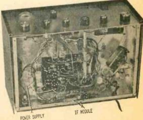
Another view of author's receiver, showing placement of module and power supply.
