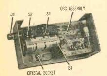
Completed perf-board assembly is mounted in chassis by attaching it to the meter terminal screws. After wiring has been checked for errors and the battery installed, Rock Rater is ready for a trial run and calibration.
