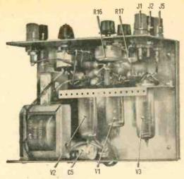
Most of circuitry is located on sub-chassis which mounts the three tubes. Nothing in circuit is critical and variations can be made.
