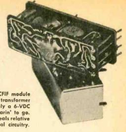
gain and three additional tuned circuits) to your receiver's IF strip, and you'll get lots of DX-making zonk. On the author's hookup to an EICO "Space Ranger," the little goody added 55 dB gain and knocked bandwidth down to about 3.5 kHz—an appreciable improvement.
