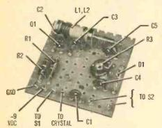
Majority of Rock Rater components are mounted on perf-board and wired following the schematic. Completed board assembly is then wired to chassis-mounted components and installed in chassis.
