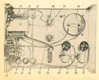
Internal layout of parts in Dynamic Duo isn't critical and can be modified to suit.
