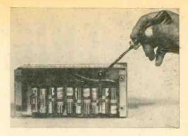
Rear apron of FETVM contains 10 batteries and coarse zero adjust control accessible through hole in rear cover.
