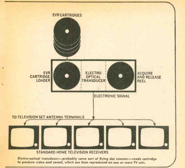
a special unperforated film, 8.75 millimeters wide. This master film is used to run off copies for purchase of EVR customers. Such copies are packaged in cartridges 7 in. in diameter and ½ in. thick—about the size of a standard reel of magnetic tape.
