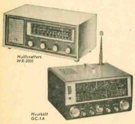
Some special types of receivers can be used for SWLing. For example, above is a deluxe table model set featuring several SW bands; below is portable transistor all-band job.
