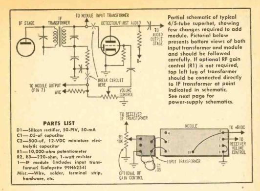
transformer feeds the detector, which, in budget receivers is usually a 6- or 12AV6.
