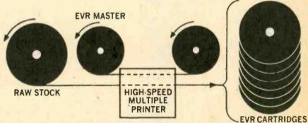
High-speed multiple printer produces multiple copies from EVR master. One twenty-minute film can be reproduced in approximately thirty seconds.
