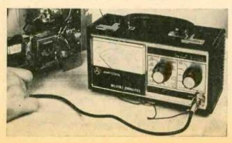
As substitute for both VTVM and AC-VTVM, the Amphenol FETVM provides the user with a substantial number of useful features at a reasonable cost.
