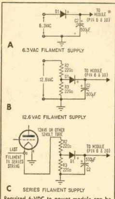
Required 6-VDC to power module can be provided by 6-V battery or one of three supplies shown above (see Parts List on preceding page for component values.)
