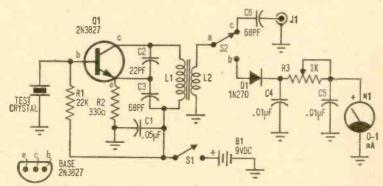
Schematic diagram of Rock Rater shows Colpitts oscillator whose output is fed to either meter M1 for rock-rating or to antenna jack J1 for channel spotting.
