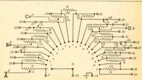
This is the schematic of the author's version of the load box; the string of power resistors, potentiometers, and series switches providing the ultimate in flexibility. At right, is the hookup employed in the knife-switch and monitoring meter circuits.
